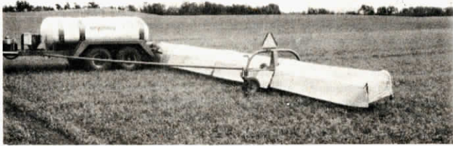
Tough nylon sailcloth covers top and back of sprayer. Flexible plastic sheets run across the front.
