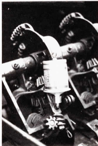
A gas-filled rubber bladder inside Perma unit forces grease into fittings, as needed.
