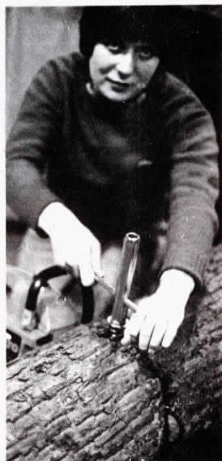
A few turns of the Uniskredge frees pinched chain saws, preventing damage.
