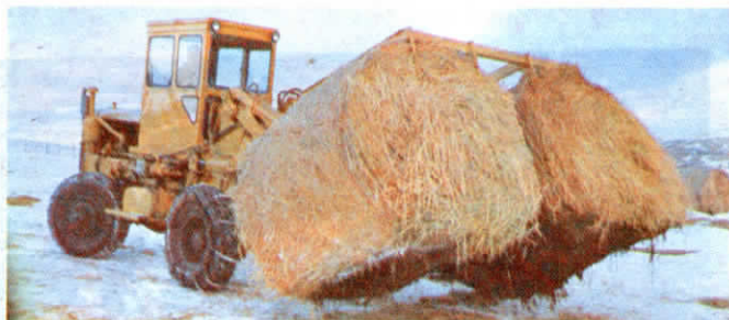
The loader's grapple fork is big enough to handle two round bales at a time.
