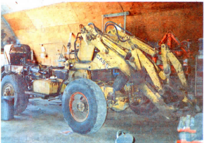
Lansdell stripped a 4-WD surplus government snowplow down to the frame, salvaged the loader from a Case 1000D crawler tractor, and mounted it on the snowplow frame.
