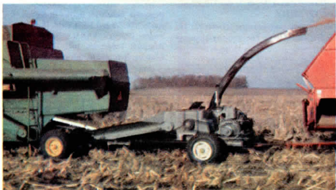
A belt conveyor carries residue from the back of the combine into the mobile hammer-mill grinder which blows the chopped-up residue into a trailing wagon.
