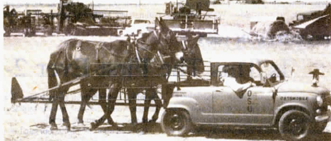
Mules are strapped into a harness that pulls against rails on either side of animals. Clark uses two sets of reins to control the team right from the cab of the cut-down car.
