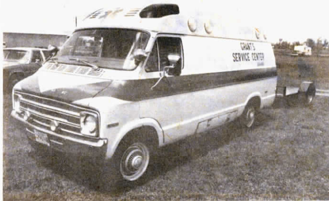
Grant Hanson makes on-farm service calls with this converted medical ambulance. Floodlights all around the outside edge of the van are used to light up jobs at night.
