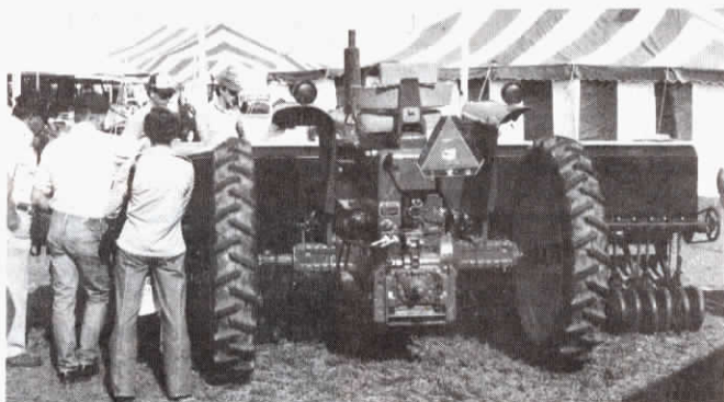
Narrow (9 in.) rims and tires were mounted on the rear of the tractor to minimize wheeltrack damage when interseeding soybeans into standing wheat.
