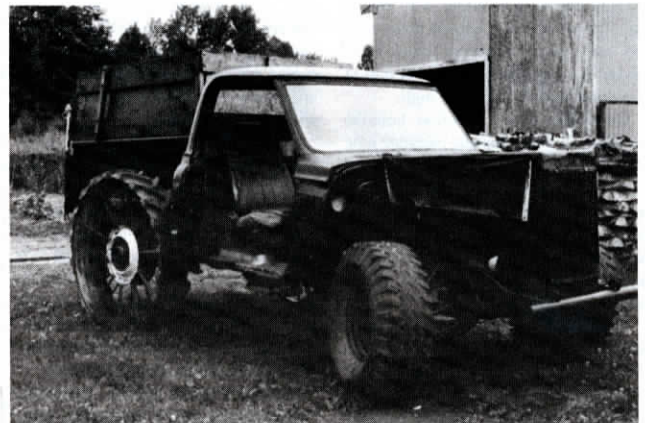
This "Timberdoodle" has steel wheels covered by rubber tread which lets it be used on highway. Hansen fitted an 8-hole 3/4-ton truck rim center to the spokes.
