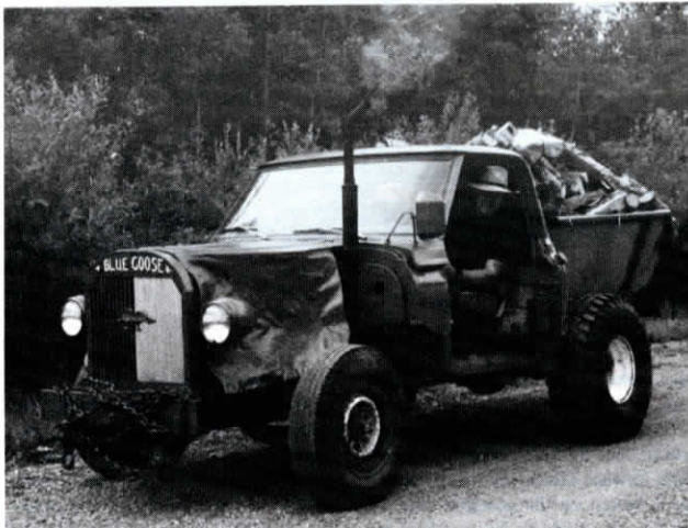
Hansen uses this rig fitted with oversize rubber tires to haul firewood.
