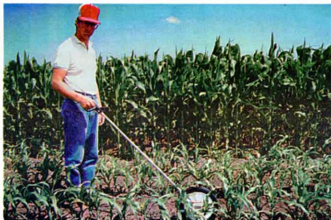
The "Space Cadet" has a 12-in. dia. rubber wheel connected electronically to a distance calculator, and a wire "stem counter". Unit is rolled alongside a row of corn.
