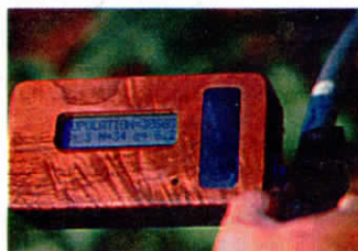
The number and location of "clicks" are recorded in a computer-driven monitor mounted on handle.
