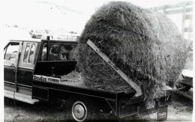
When not in use, arms fold down on sides of flatbed.
