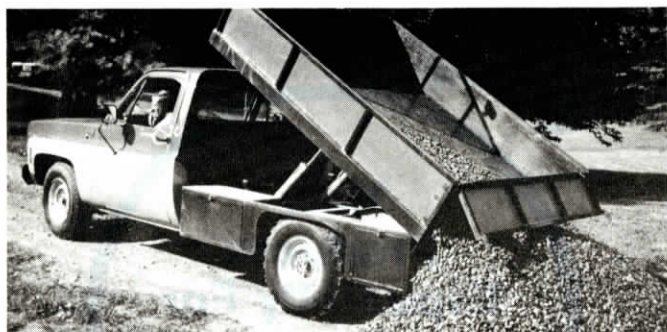
Two 2½-in. hydraulic cylinders, powered by power steering pump, can easily dump 6,000-lb. payloads.
