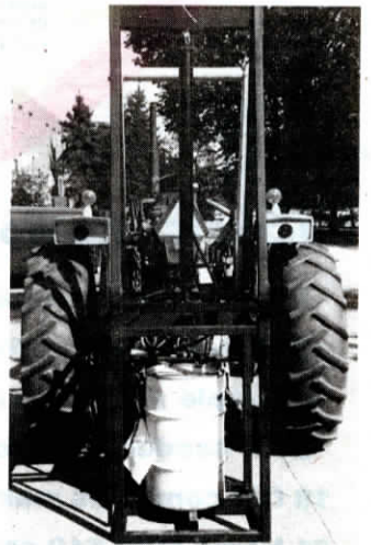
The 3-pt. mounted barrel crusher uses a cross-shaped crusher mounted on a hydraulic piston to flatten the barrel.
