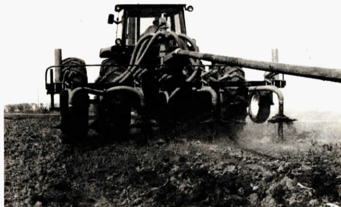
Shanks, 24 inches wide, inject manure 4 to 6 inches into the soil.
