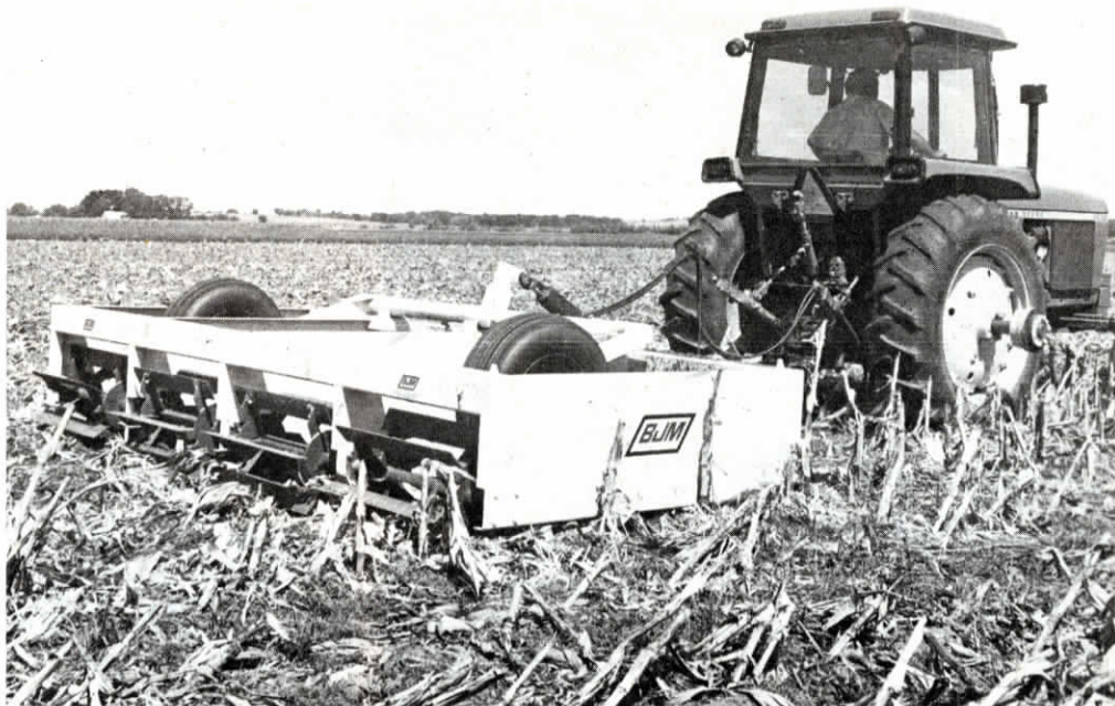
A lot of weight (2600 lbs.), plus speed, combine with reels front and back to pulverize the stalks.
