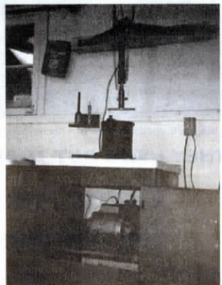
Brodt used swather and combine parts to make sausage press.
