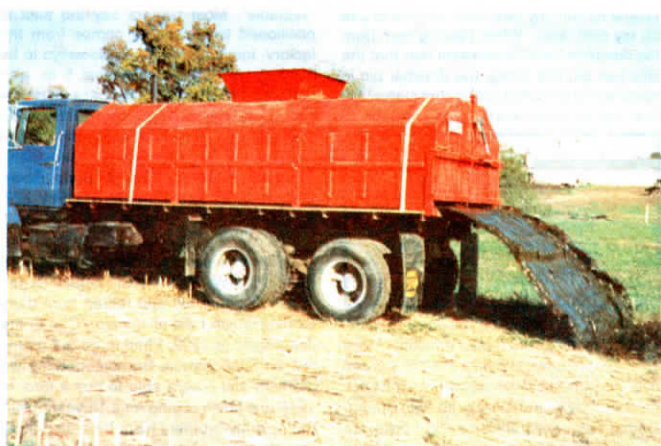
The 3,400-gal. fiberglass tank mounts on the bed of any tandem axle truck or it'll slide inside a truck box. A linear actuator activated by a toggle switch in the cab raises a rear discharge gate that unloads manure across the full width of the tank.
