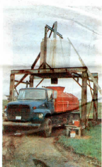
This 2,250-gal. overhead tank quick-fills the spreader in just 55 sec.
