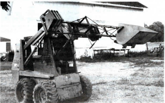
"Side Kick" quick-taches to loader so Cooley can quickly drop it off when he's done cleaning out bunks. He uses the side-mount bucket every day.
