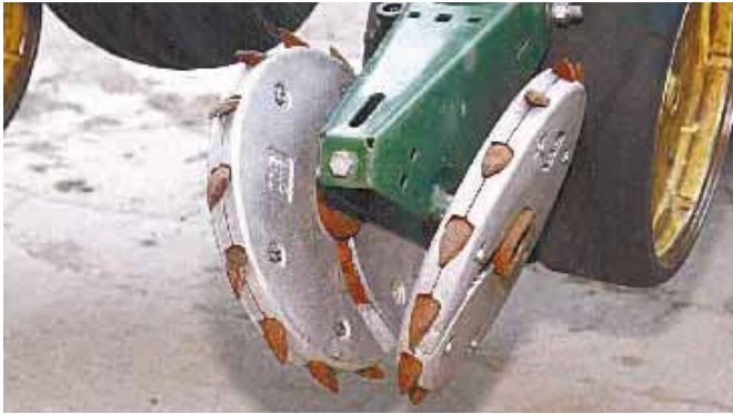
System uses spoked wheels that are partially covered by 11 1/2-in. dia. aluminum plates. Plates cover one or both sides of closing wheels, depending on soil conditions.
