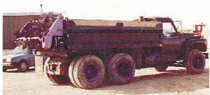
Self-contained kit consists of heavy-duty drag chains, aluminum slats, and beater bars which slide into truck as a single unit. Plumbs into truck's existing hydraulics.
