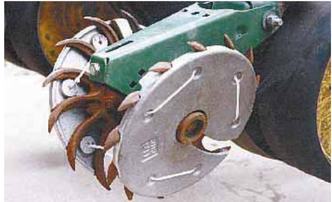
Half-section plates are held on by metal clips and can be fastened to either the inside or outside of the wheels, depending on soil conditions.
