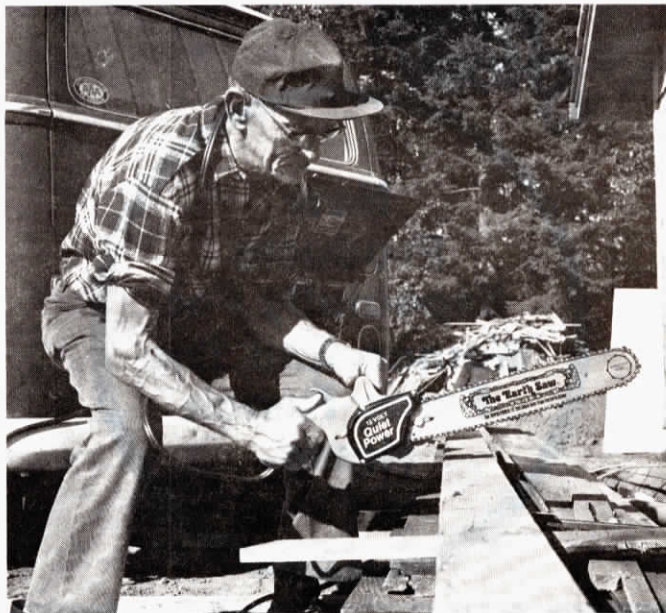
Battery-powered Earth Saw weighs 6 lbs. and cuts through logs up to 28 in. in dia.
