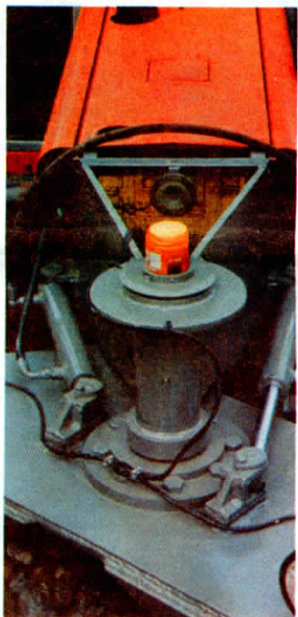
Cylinders on either side of king pin turn big front wheel. They're plumbed into tractor's existing power steering.
