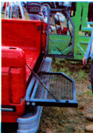
You can lift up either side of tailgate when it's down.
