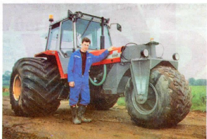
Converted Massey 690 no longer leaves deep wheel tracks on Atkinson's heavy clay soil, improving seeding accuracy when planting crops.
