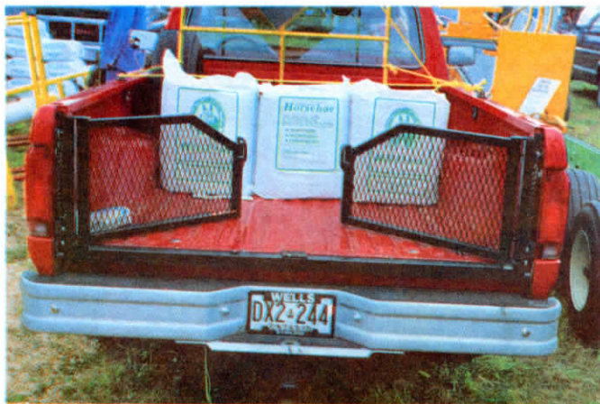
Air-through tailgate opens at center for easy access to cargo and makes it easy to step up into truck box. It also locks at center to open like a normal tailgate.
