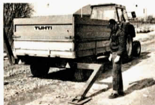
Leg in foreground is shown in "lift" position. When not being used, insertable legs ride in up-raised position, shown by leg on left.
