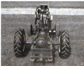
Gearbox belt-drives dual gear boxes. (Photo shows seat removed.)
