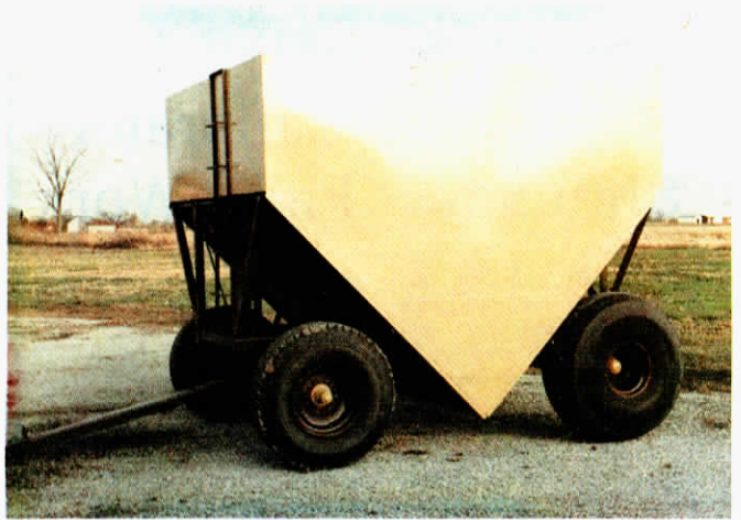
The bottom of the steep-sloped box is indented to fit over the center beam on a 4-wheel wagon gear.
