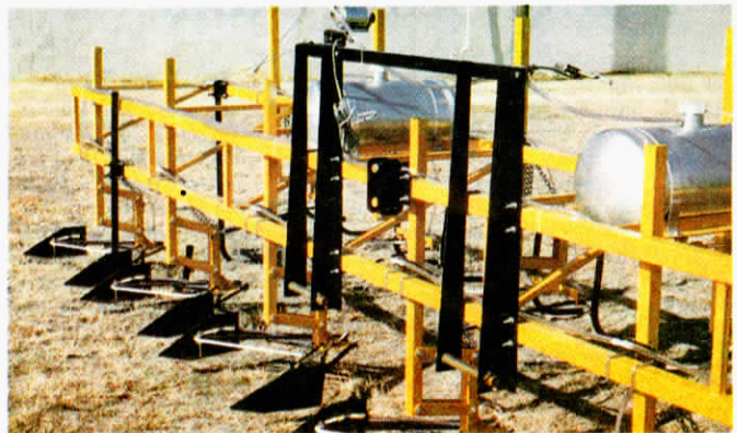
Between-the-row rope wicks eliminate the need for cultivators, says the manufacturer of this soon to be introduced Vogel between-row wick weeder.
