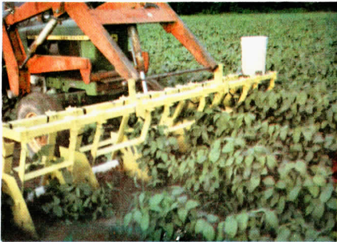
Wedge-shaped wicks fit right down between the rows, separated from the crop by row shields.
