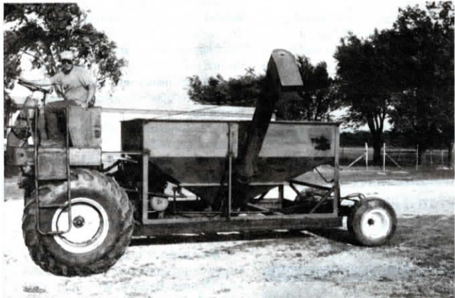
The Depenbusches used front axle and drive train off a Super 92 Massey Ferguson combine with 28-in. tires. Rear axle is off a Massey Ferguson 410 combine.
