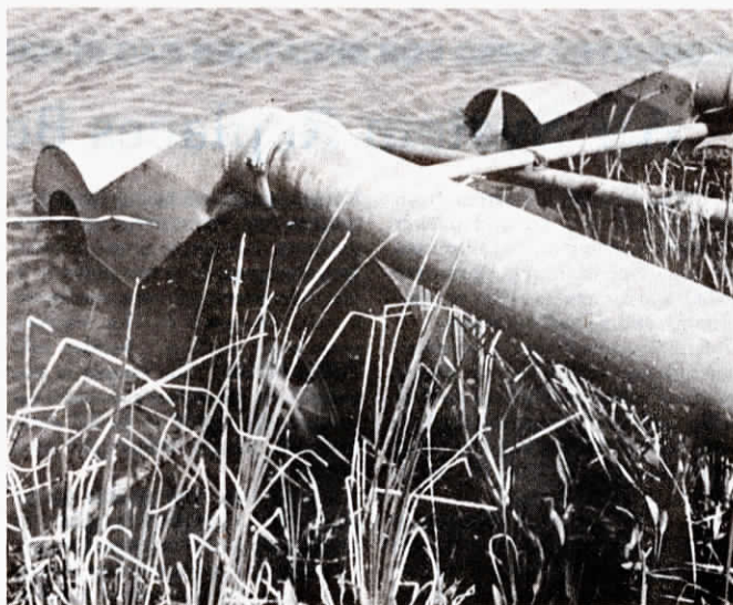
Portable pump is backed into water so its wheels and impellers drop below the water surface. Photos courtesy Texas Farmer-Stockman Magazine
