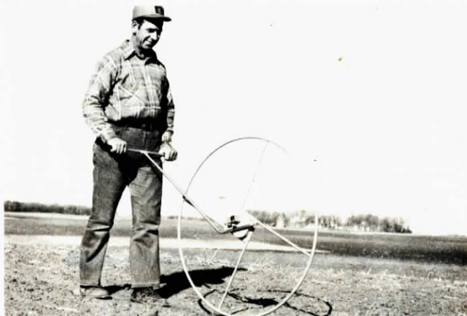
The 10 ft. tubular steel wheel accurately measures plowed ground and other rough terrain.
