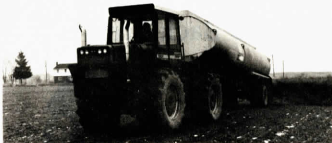
Salvaged oil tanker is equipped with a Calumet "Slinger" in back, and is pulled by a 5th wheel mounted on the back of the tractor.
