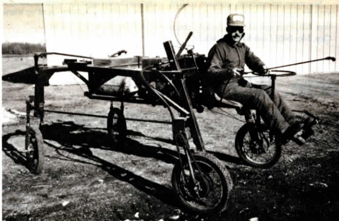
You steer the bean buggy with one hand and spray with the other.
