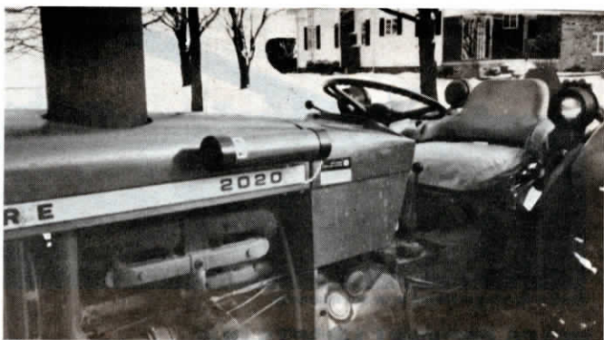
Waterproof canister for storing instruction and parts manual can be mounted where most convenient.
