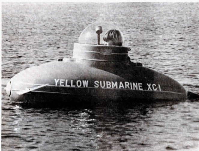
Thomas Taylor's battery-powered submarine dives to 300 ft., running at speeds up to 5 mph.
