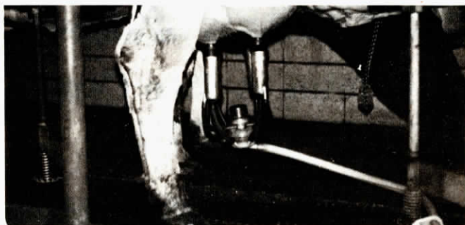
Bodmin Nu-Pulse milker uses .8 cu. ft. of air per min., versus 10 cu. ft. for conventional milkers. Note the "one hose" hookup. Retail for $314 per unit, including the washer.
