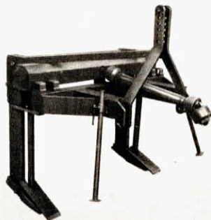
Front shoe, and vertical shaft hooked to it, moves up and down at rate of 250 2 in. strokes per min.
