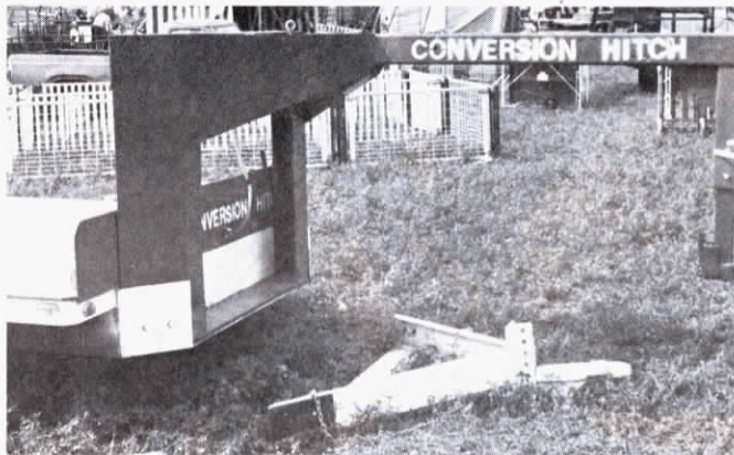
Conversion Hitch lets you switch from gooseneck to straight hitch in minutes.
