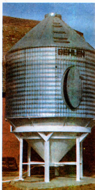
Bocat's hopper bottom cones hold right at 250 bu. Bottom end of the cone is 20 in. off the ground.
