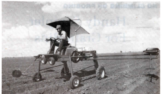
Belts driven by rear mower tires power new bean rider.
