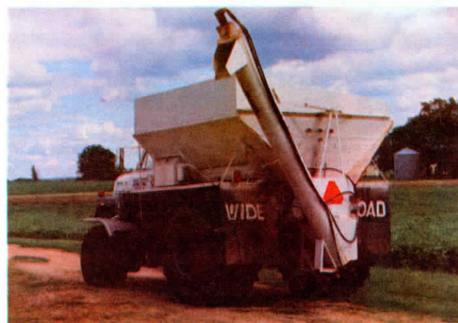
Thompson removed spinner spreaders on back and replaced them with a 12-in. dia. auger that's powered by hydraulic motor.
