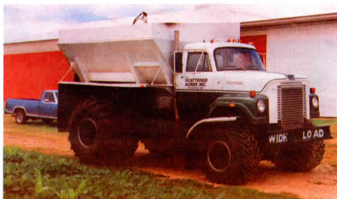
Thompson raised the sides of hopper with sheet metal, adding 3 ft. on one side and 1 1/2 ft. on other side so combine's unloading auger can reach over it.
