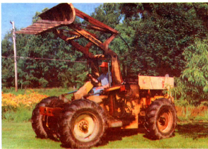
Hart's built-from-scratch tractor was built with two 2-speed truck axle rear ends.
