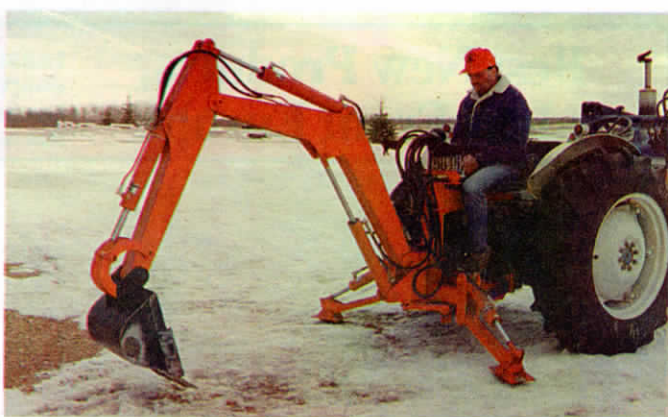
Giasson's 3-pt. mounted digger mounts on any Cat. I or II tractor with hydraulics, or a hydraulic power pack can be added.
