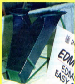
Chute bolts on in place of two steel plates at bottom of tank.
