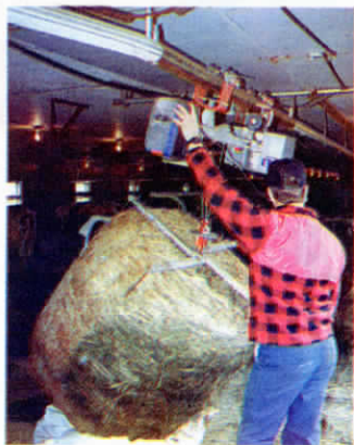
To load a bale, you insert a steel rod through its center and attach cross arms to top and bottom. A winch lifts bale up.
