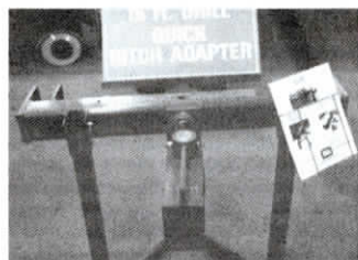
New hitch bolts provides better weight transfer between tractor's drawbar and drill's standard drawbar-type hitch.
