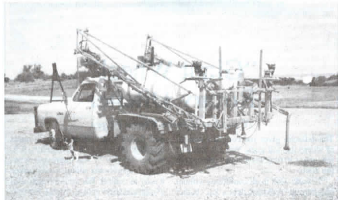
DeBruycker modified his 1983 Dodge 350 1-ton pickup, mounting new 24-in. wide, deep lug flotation tires and a 500-gal. tank and 60-ft. Blumhardt boom on back.
