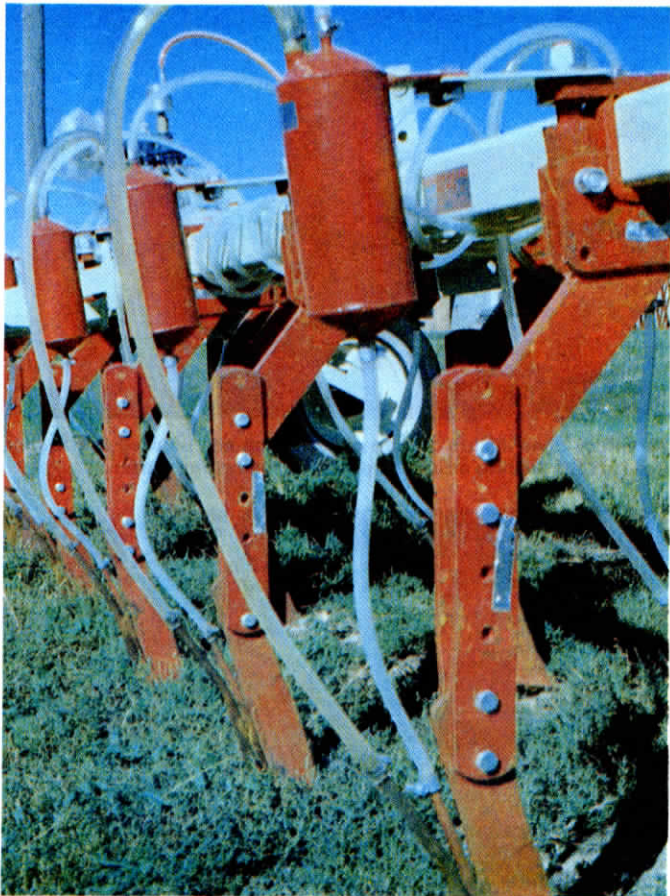
Individual row units convert anhydrous to liquid. The new concept takes less power than direct application of \text{NH}_3 , there's less leakage loss, and it's safer to apply, says Louis Siebert.
