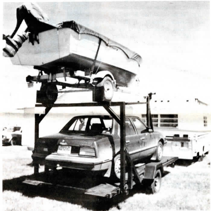
A 2-way power winch loads the boat onto the upper half of boat-car trailer.
