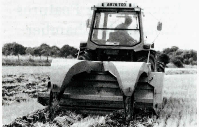
Parmiter straw chopper blows straw into slots made by rear-mounted subsoiler shanks.
