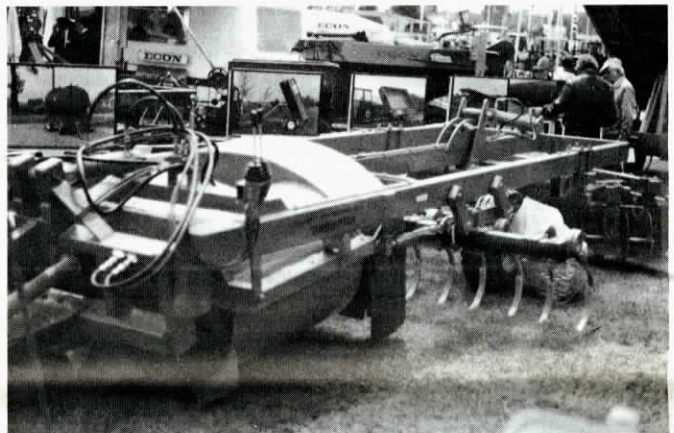
Whirling blades in up-front "Turbovator" drums suck straw off ground, chop it, and then blow it out the back where it's incorporated by spring tines and discs.
