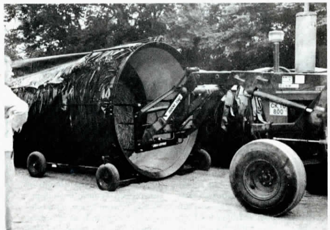
Ammonia is automatically injected into each bale through bale spears on tractor loader.
