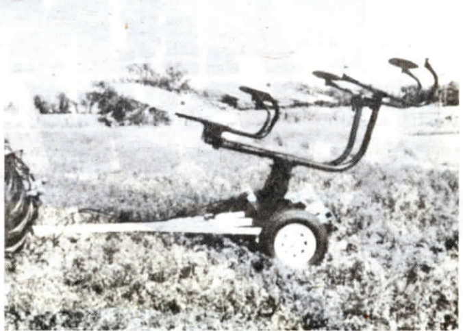
Trolley converts V-rakes from 3-pt. mounted to pull-type. One cylinder folds rig from raking to transport position.
