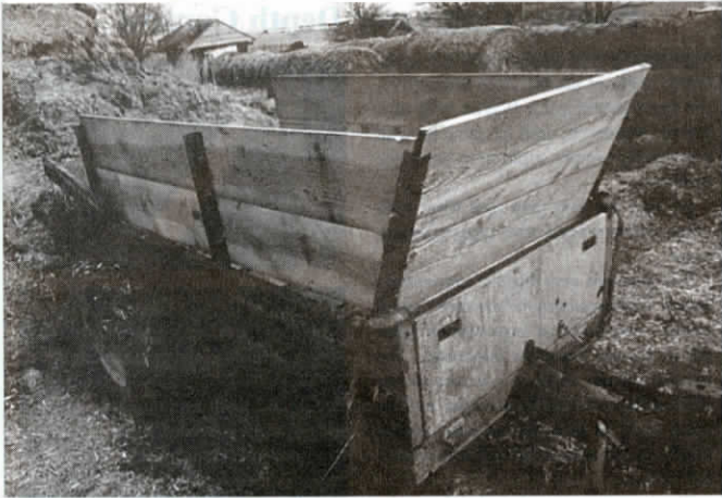
Gogerty made feed wagon out of worn out Deere 34 manure spreader.
