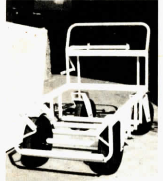
Rollers make it easy to slide animal onto the dead sow cart.
