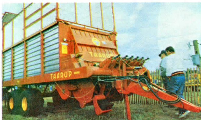
Up-front chopper cuts, chops and feeds haylage up into wagon, which has 40 percent more capacity than conventional wagons because material is compacted as it's loaded.
