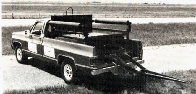
Hydraulic spike loads the feeder and can withdraw to pick up a second bale.
