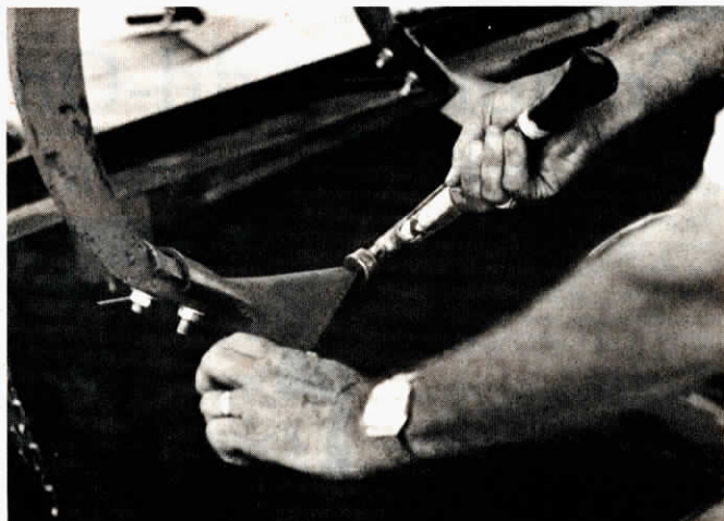
After an adaptor clip is bolted to cultivator shank, sweeps can be changed quickly with only a hammer.
