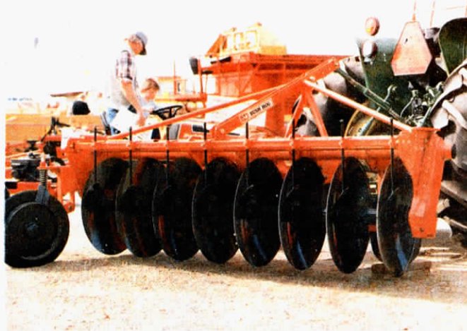
Machine's 25-in. dia. discs till to a depth of 10 in.
