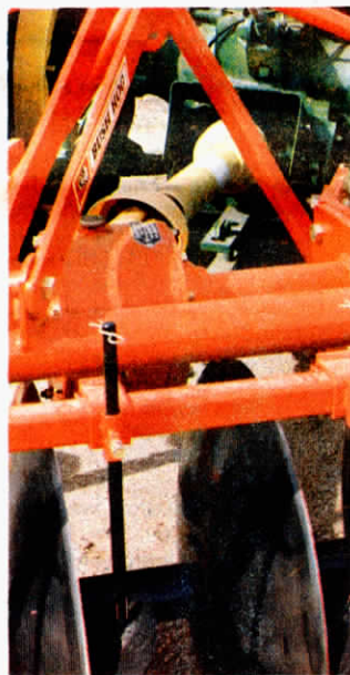
Disc uses just one-third the power required by a similar size plow.
