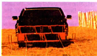
Trailer has five compartments - three on top and two on bottom - each holding a spool of barbed wire.
