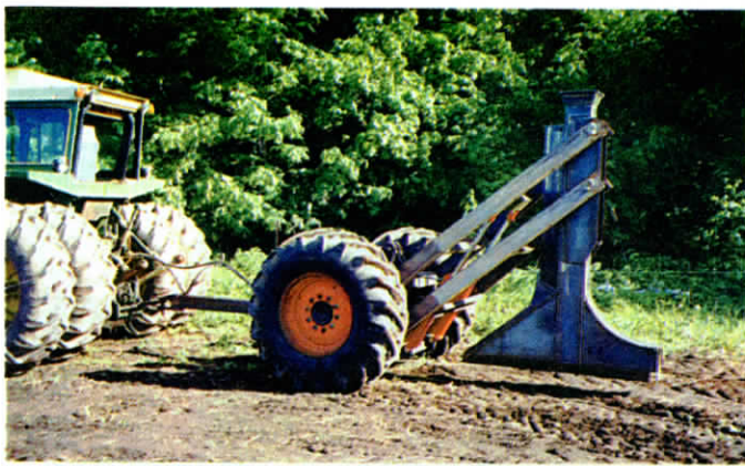
Tile plow pulls behind wheeled carrier made out of combine axle.
