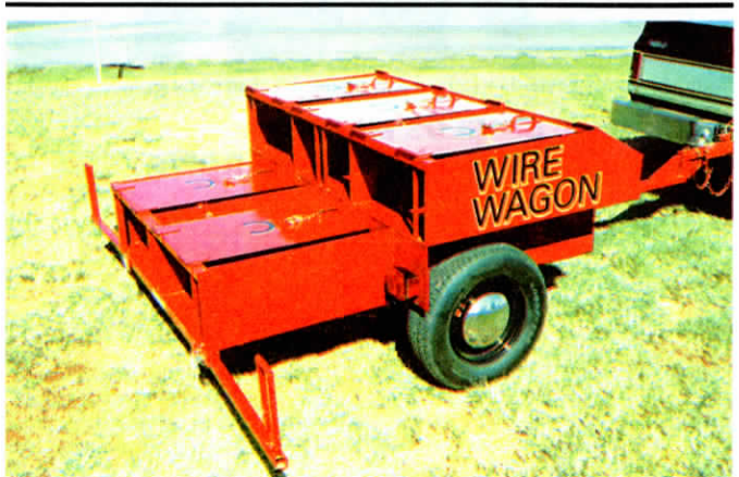
Two-wheeled trailer has a ball hitch so it can be pulled with tractor or pickup.
