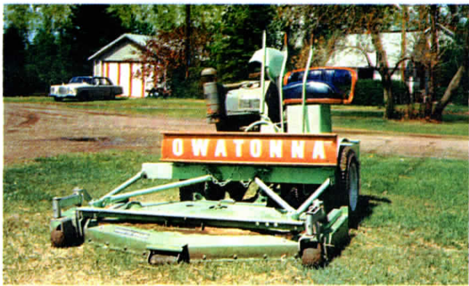
Reinhardt turned an Owatonna swather into a zero-turn 60-in. riding lawn mower by "miniaturizing" it and adding Deutz-Allis belly-mount mower in front.
