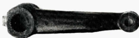
The company welds a block to the side of the head of the old arm, then cuts a slot through the block and head.
