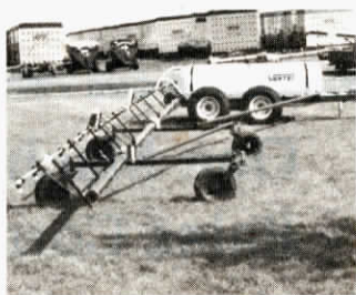
New sprayer has quick fold booms, and a low profile tank with molded in baffles.
