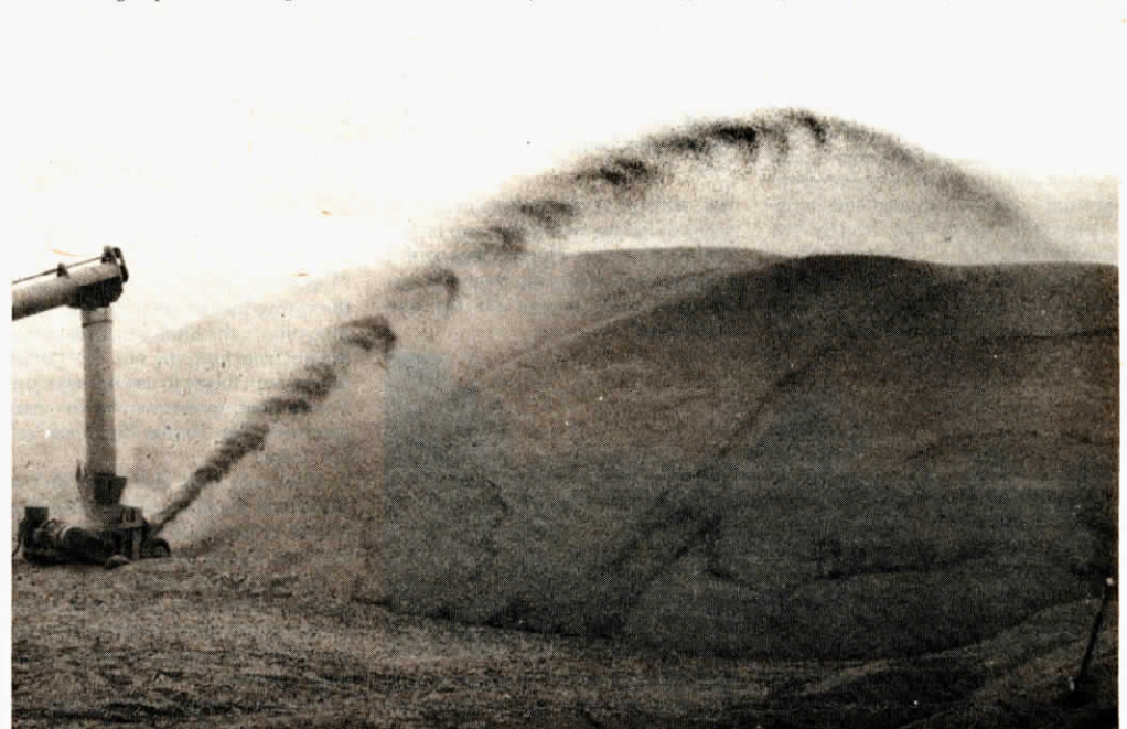
"Slinger" will throw grain into a pile up to 40 ft. high and 200 ft. in dia. It's powered by a 5 hp electric motor.
