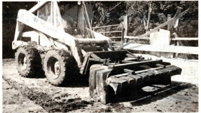
Half-tire scrapers fit chore tractors and skid steer loaders. Optional scraper bar drags manure out of corners.
