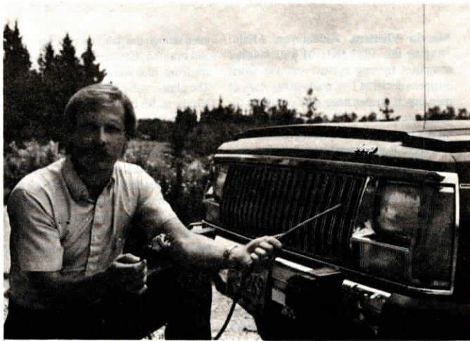
Power cord consists of 17-ft. long cord (30 ft. for trucks) wound onto a retractable reel mounted under the hood.
