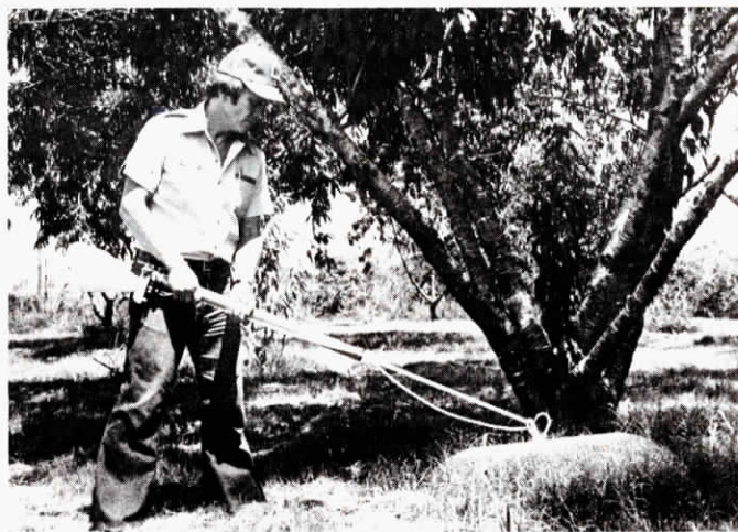
With Herbi sprayer held approximately 8 in. from target weed, with no wind, the 4 ft. swath falls 2 ft. either side of atomizer nozzle.
