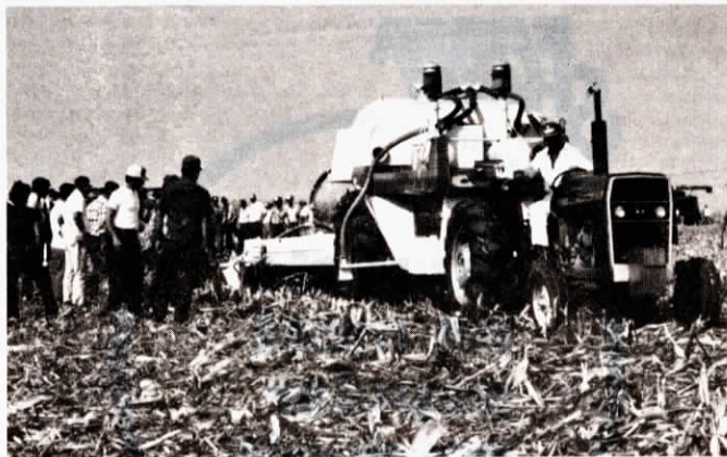
A 60 to 70 hp tractor pulls the Maxicultivator, which has its own 314 hp power unit.
