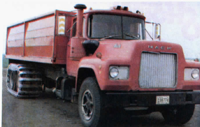
Loegering Mfg., Casselton, N. Dak., makes tracks for straight trucks, in addition to combines, tractors or skid-steer loaders.
