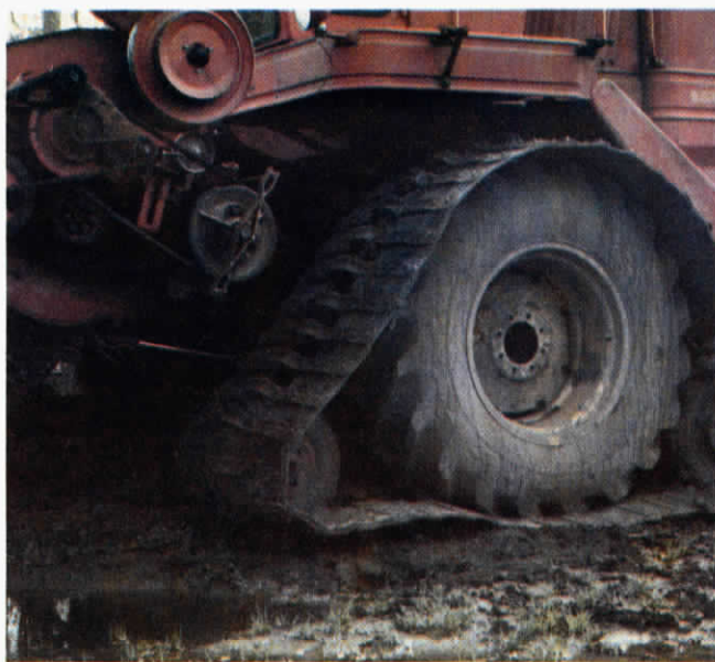
Above photo shows do-it-yourself tracks designed by Ag Engineers at Canadian Dept. of Agriculture, Edmonton, Alberta. Building a set takes about 100 hrs. and $1,000 worth of materials. If you'd like a set of plans, send $3 to: Combine Tracks, c/o FARM SHOW, Lakeville, Minn. 55044. Make check payable to Combine Tracks.
